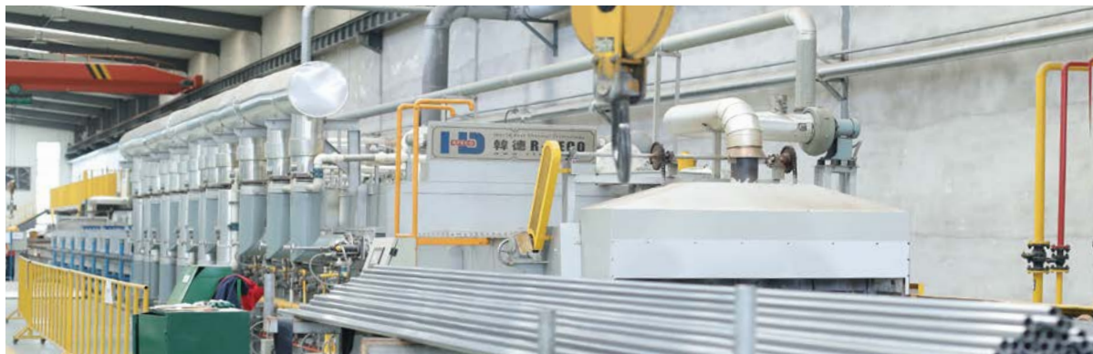
Korean HANDUK roller hearth type continuous anaerobic annealing furnace
