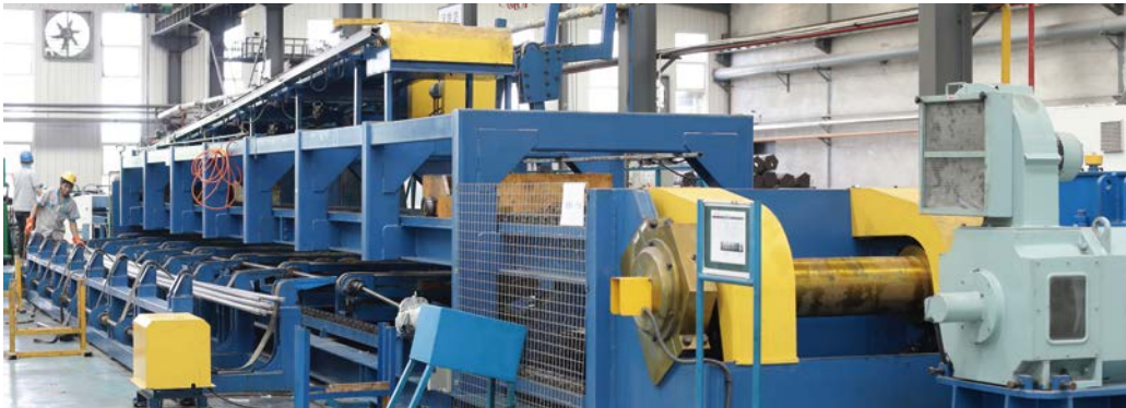
Korean triple drawing bench line
