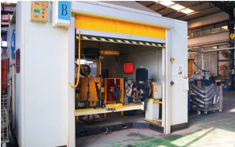
Robotic Welding Machine
